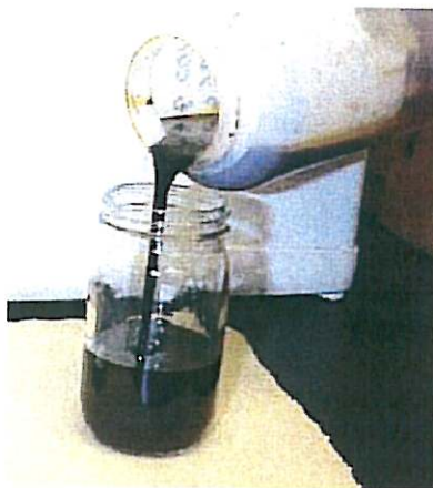
Figure 3-8. Bio-oil Produced from Pyrolysis (Source: Iowa State University).
