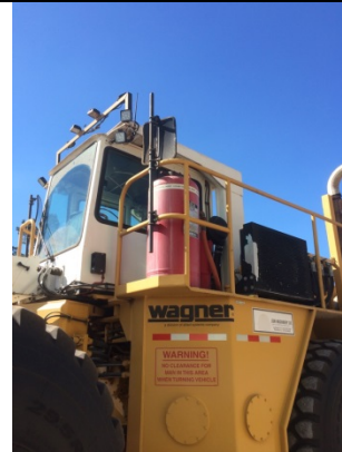
Detail: Fuel pile equipment with automatic fire suppression
