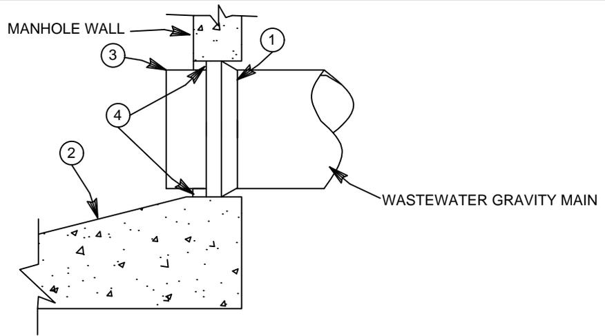
**NEW PREFABRICATED INVERT SANITARY SEWER MANHOLE**
