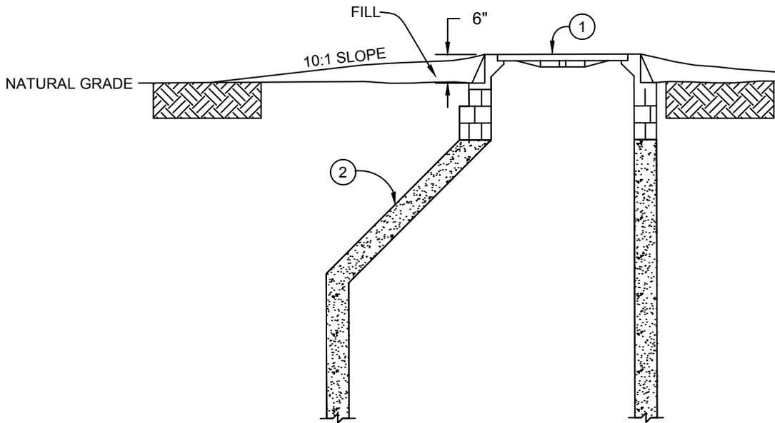
NOTE: WHEN MANHOLE IS OUTSIDE PAVEMENT, THE RIM ELEVATION SHALL BE 6" ABOVE NATURAL GRADE, WITH FILL ADDED FOR A 10:1 SLOPE TO NATURAL GRADE.
